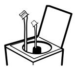
Loosely load clothes no higher than the top row of holes in the washer basket. The water level should just cover the clothes.
