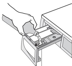
Pour fabric softener into the compartment marked (must not exceed the «MAX» mark in the drawer).
