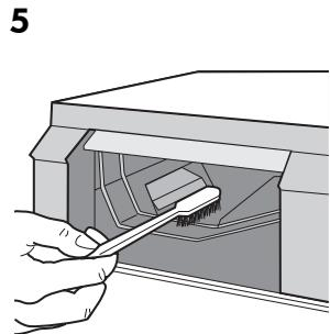
To aid cleaning, remove also the top part of the additive compartment.
