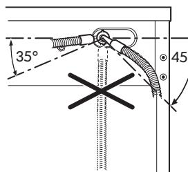
Turn the inlet hose to the left or the right to suit the installation. Tight the locknut correctly to prevent water leaks.
