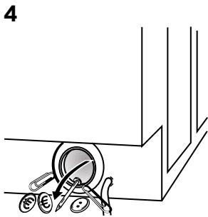
Place a container close to the pump (A), to collect any spillage.
