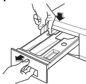
To remove the drawer, press the catch downwards and pull it out.
