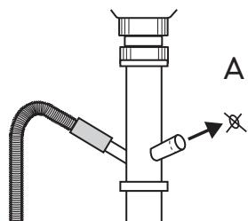
If you connect the water drain hose to a water trap under the sink, remove the plastic membrane (A). If you do not remove the membrane, detergent residue and clothes fluff can cause a blockage in the drain hose spigot.
