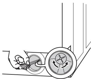
Use a pencil to check whether the pump wheel right at the back of the pump housing can turn. (It is normal for the pumping wheel to turn jerkily.) If the pumping wheel cannot be turned, please contact the After Sales Service.
