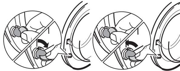
To activate this device, rotate the button clockwise (without pressing it) inside the door until the groove is horizontal. If necessary use a coin.
