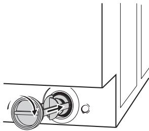
Put the cap back on the emergency emptying hose and place the latter back in its seat. Screw the pump fully in.
