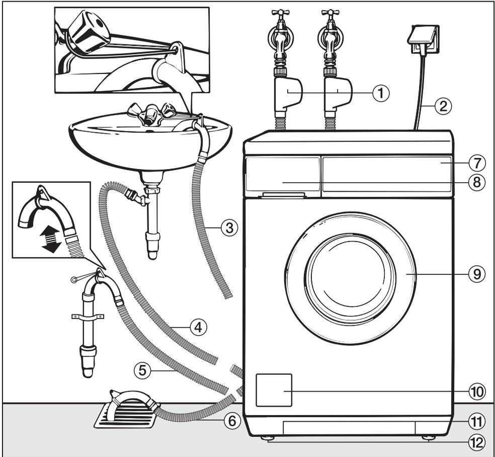
① Inlet hoses with "Waterproof system" for cold water and hot water connection
