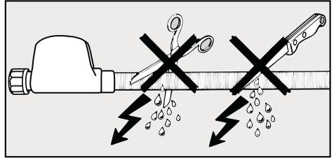
**The protective sleeve of the hose must not be damaged or kinked.**
