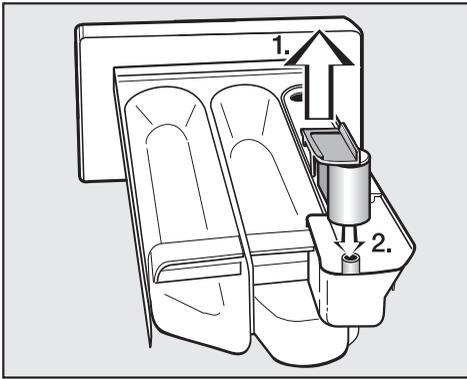
1. Remove the siphon from compartment
