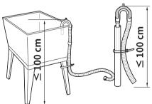
If the drain hose is too long, do not force it back into the appliance. This will cause abnormal noise • Connect the elbow bracket a within **10 cm** of the end of the drain hose.
