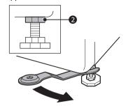
4 Check if all lock nuts at the bottom of the appliance are secured properly.
