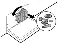
After cleaning the drain pump filter, carefully reinsert the filter and screw the drain cap back in clockwise carefully to avoid cross threading and leakage. Reinsert the plug back into the drain tube and place the tube into its holder.
