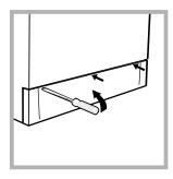
1. using a screwdriver, remove the cover panel on the lower front of the Washer-dryer (see figure);
