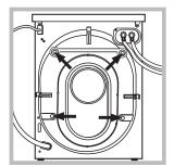
3. Remove the four protective screws and the rubber washer with the respective spacer, situated on the rear of the appliance (see figure).
