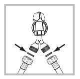
1. Connect the supply pipe to the water mains using a gas 3/4 attachment, fitting the rubber gasket and the filter supplied with the appliance and ensuring that they are fimly tightened to the taps. The water supply marked
