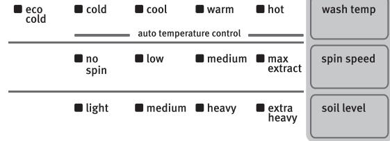
Once you select a cycle, the default settings for that cycle will be lit. Press the Modifier buttons to change the Wash Temp, Spin Speed, and Soil Level, if desired. Not all settings are available with all cycles.
