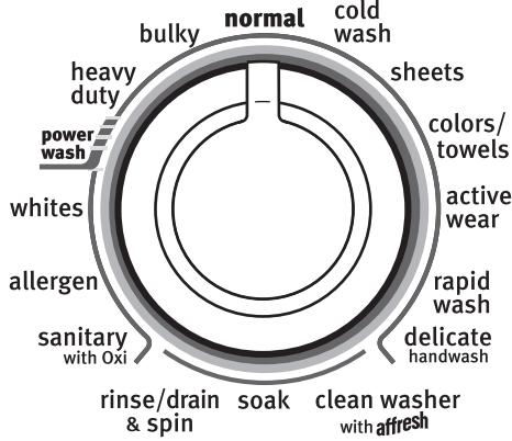
Turn cycle knob to choose your wash cycle. Estimated Time Remaining will light up with a cycle time. You may notice time adjusting during the cycle. This is normal.
