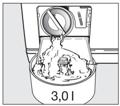
■ Unscrew the drain filter lid until water runs out.
