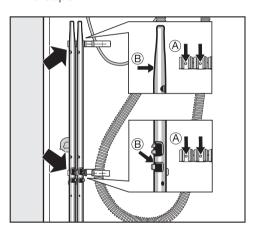
Secure the transit bars to the back of the washer-extractor. Make sure that holes
