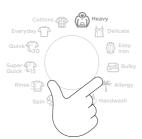
Select your desired wash cycle by turning the Control Dial. The wash cycle icons will illuminate as you turn the dial showing which cycle is selected, along with the default wash cycle settings.
