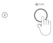
The cold **WASH TEMP** icon will flash on and off. This is the default setting, where the machine uses the internal heater to heat the water to 20°C.
