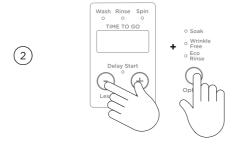
Press MORE  $\pm$ , LESS – and OPTIONS buttons together for three seconds, dEF will appear on the screen and the washer will beep.
