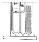
If you wish to use the **PRE WASH** option, liquid or powdered detergent only must be placed in the pre wash detergent compartment on the right side of the drawer, marked with a (1).
