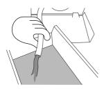
Unhook the pump outlet hose and pull it out (about 150mm). Remove the plug and allow any water (approximately 250ml) to drain into a shallow dish.
