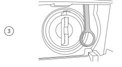
Pull the door release tab down from the ring. Use a screwdriver tip, pen or key to get a good grip.
