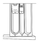
Detergent is added to the main wash compartment on the left side of the dispenser drawer marked with a  $\widehat{(II)}$ .
